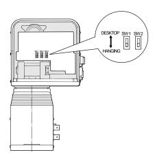
If the pan/tilt head is connected to the control panel with a cable longer than 300 meters, set the cable compensation switch on the pan/tilt head to the ON position in advance. If the distance between the pan/tilt head and the control panel is shorter than 300 meters, keep the switch in the original position (OFF).
